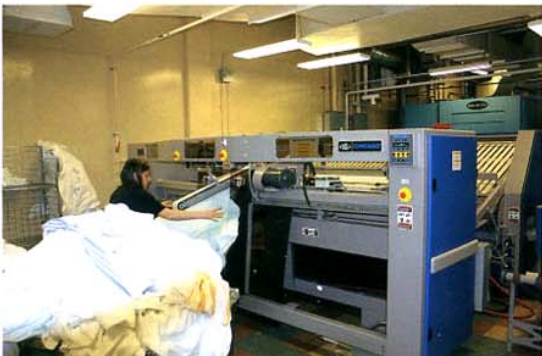
Below: Shelly Willis feeds flannel sheets into the Chicago Edge blanket folder. Right: from left, George Dunn, Cody McLure, Andy Hurry and Jason Condon sort incoming soiled work into slings.
